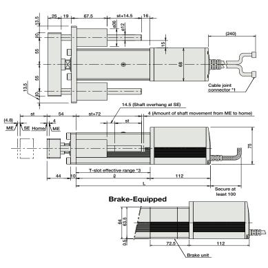
$^{\star}$  Compared to the standard model, the brake-equipped model is longer by 72.5mm and heavier by 0.9kg.
