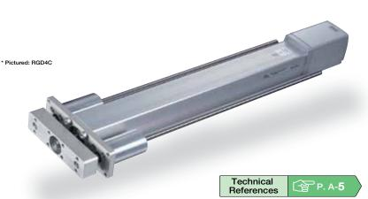
(1) When the stroke increases, the maximum speed will drop to prevent the ball screw from reaching the critical rotational speed. Use the actuator specification table below to check the maximum speed at the stroke you desire.
