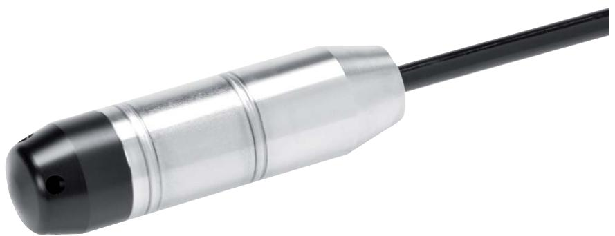
The pressure transmitters of type 681 with piezoresistive measuring elements have compensated, calibrated and amplified sensor signals which are available as standard voltage or current outputs.
