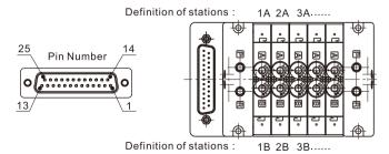
Note: Gauge number of cable connecting to D-Sub pin No.13(COM) must be≤22AWG
