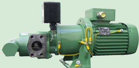
e.g. binders pump (resins) according to ATEX with double GLRD (mechanical seal), quench recipient and temperature control
