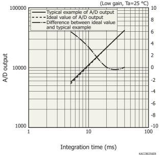
A/D output is the output with dark output is subtracted when light is input. The difference between the ideal value and typical example contains a measurement error. The smaller the A/D output, the larger the measurement error.
