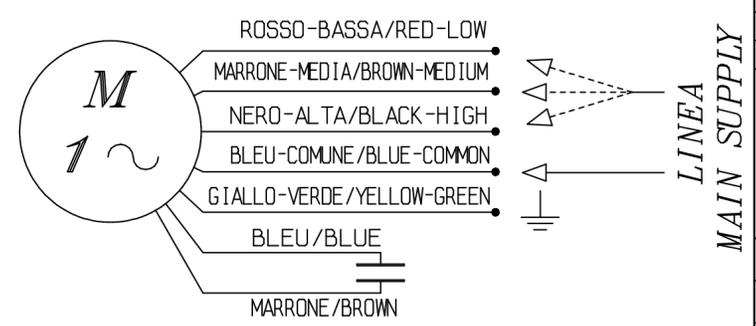
MOTORE CON PROTETTORE TERMICO
