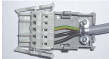
Fix the upper part (part **B**) of the strain relief housing by snapping it onto the lower part.
