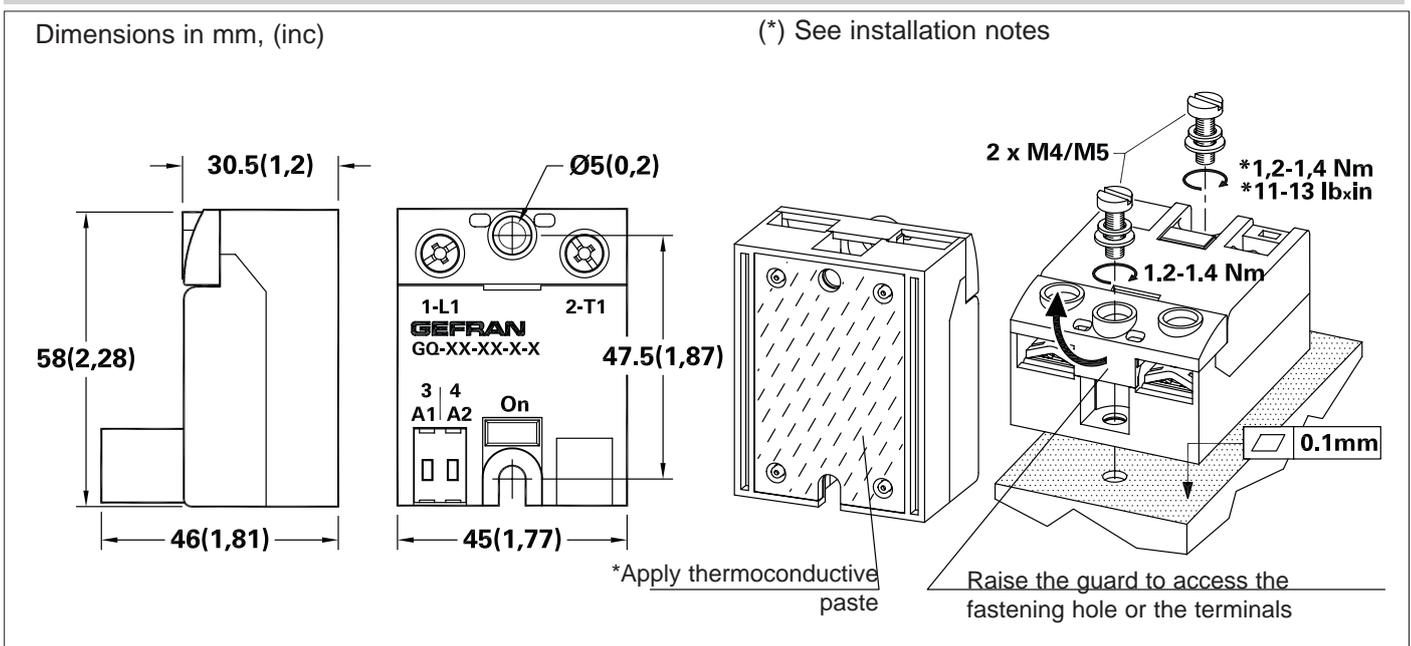
spread 1 gram of thermoconductive silicone paste (we recommend DOW CORNING 340) on the dissipative metal surfaces of the module.
