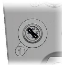
Fig. 18: Conductive rubber band in connection socket 1
