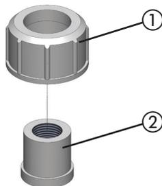
Fig. 13: Cemented connection
