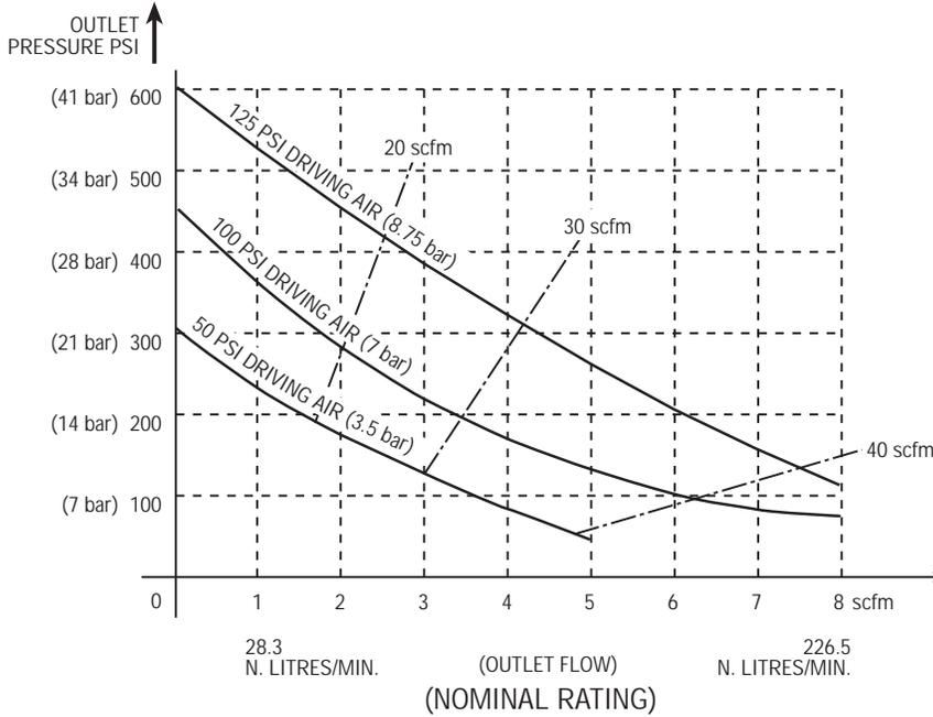
Solid lines indicate approximate flows at various driving air pressure. Dotted lines indicate air consumption in scfm.
