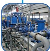
Shell & Tubes heat exchangers are used for the cooling of hydraulic circuits and are normally installed in return lines.
