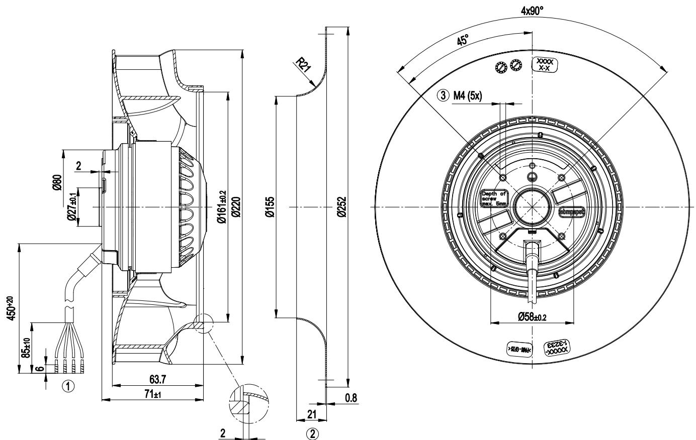
1 Connection line silicone 4G 0.5 mm<sup>2</sup>, 4x brass lead tips crimped
