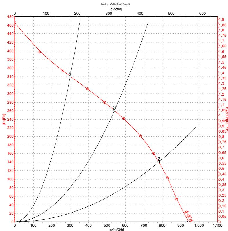
Air performance measured as per ISO 5801 Installation category A. For detailed information on the measuring set-up, please contact ebm-papst. Suction-side noise levels: LwA measured as per ISO 13347 / LpA measured with 1m distance to fan axis. The values given are valid under the measuring conditions mentioned above and may vary according to the actual installation situation. With any deviation from the standard set-up, the specific values have to be checked and reviewed with the unit installed.
