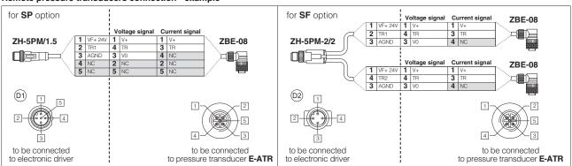
Note: pin layout referred to connector view
