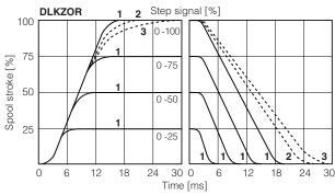
(\*) Response time is represented only for 0-100% step; for intermediate steps, the response time increment of presets 2 (balanced) and 3 (smooth) with respect to the preset 1 (dynamic) is proportional to the step amplitude of the reference input signal
