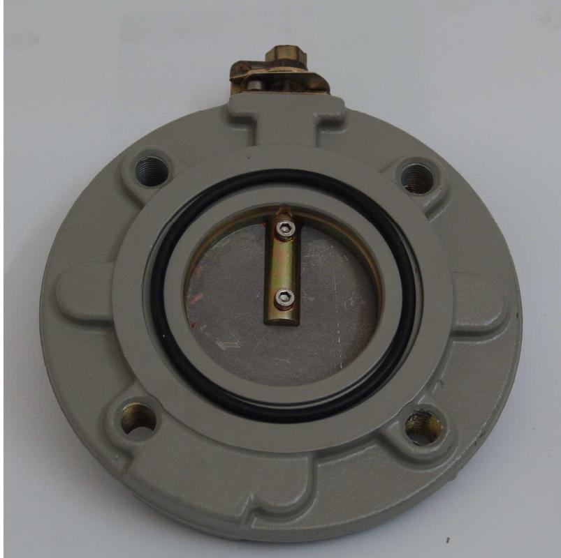
This kind of valves, metal to metal sealing, are used on power transformers with the scope to allow the disconnection of the Buchholz relay from the conservator or from the cover; they are preferred to the conventional gate valves for their compact overall dimensions in the direction of the oil flow.
