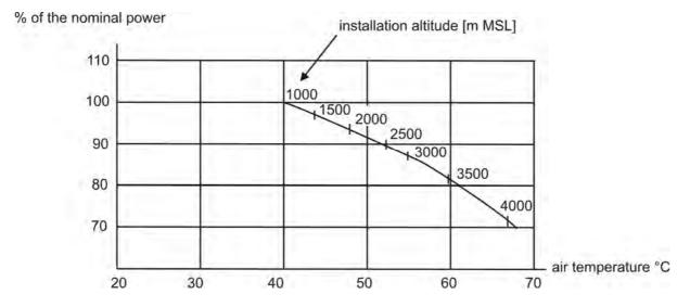
Check the air temperature and the installation altitude separately. Should there be differing air temperatures and installation altitudes concurrently, the factors concerning available nominal power need to be multiplied.
