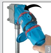
Rotating the 'dead' plug 30° counterclockwise closes the safety shutter and frees the plug to be withdrawn from the receptacle.
